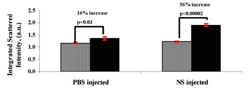
**Figure 4.** Quantification of OCT images shows a significant increase in intensity of images of tumors from mice with systemic nanoshell injection. Normal muscle tissue is shown in the blue bar while tumor tissue is shown in the black bar. Values are average  $\pm$  SEM; p values are shown.
