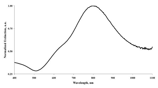
Figure 1. Extinction spectra of nanoshells used in this study. Nanoshells are 143 nm in diameter with a core of 119 nm and a shell thickness of 12 nm.
